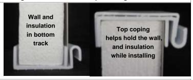
The insulation comes in sections and is notched on one side, this side is to be installed to the inside of the pool, against the wall. When placing insulation in start in the middle of the skimmer section slightly curve to the track with your hands, placing bottom in first.
