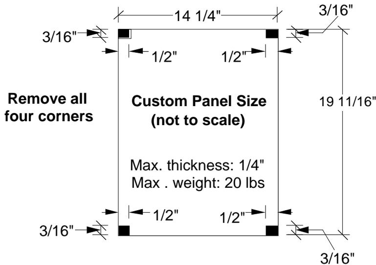
For panels thicker than 1/4", reveal is 5/8" on all sides if owner-supplied handle is used; 2" in the area of Marvels clip on handle if it is used.
