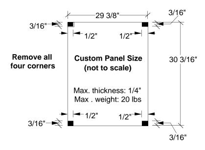
For panels thicker than 1/4", reveal is 5/8" on all sides if owner-supplied handle is used; 2" in the area of Marvels clip on handle if it is used.
