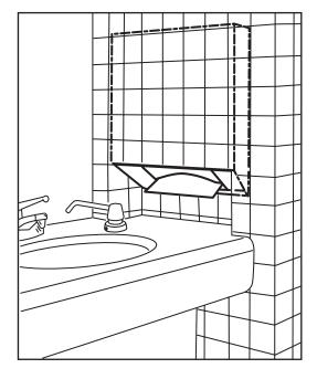
Furred mirror installation (figure 2) overhanging a bank of lavatories permits use of a full-depth vanity counter, a mirror brought conveniently close to the user, and towel dispensers above each bowel or between each pair. This arrangement also conforms to universal access codes which have height limitations that often prevent the conversational placement of both a mirror and recessed towel dispensers above the backsplash.
