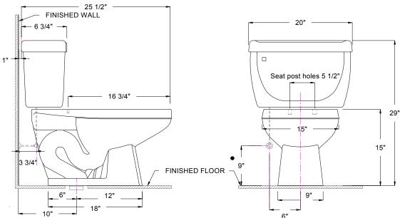
Fixture dimensions meet ANSI/ASME standards A112.19.2M, A112.196M requirements. These measurements are subject to change or cancellation. No responsibility will be assumed for use of superseded or voided pages. Dimensions shown for location of supply are suggested.
