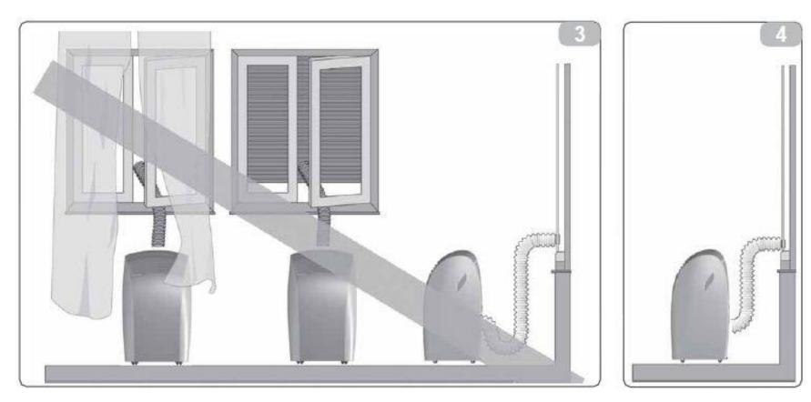
Ensure curtains or other objects are not obstructing the air inlet filters. (Fig 3)
