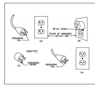
**WARNING**: This heater is for use on 120 volts. The cord has a plug as shown in A. An adapter as shown in C is available for connecting three-blade grounding-type plugs to two-slot receptacles. The grounding lug extending from the adapter must be connected to a permanent ground such as a properly grounded outlet box. The adapter should not be used if a three-slot grounded receptacle is available.
