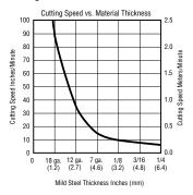
Note: The rating is based on 10 IPM because this is the minimum speed at which the operator achieves a smooth, steady cut when using a hand-held torch.
