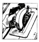
7. Slate tile can be easily cut with a wet saw using a diamond blade
