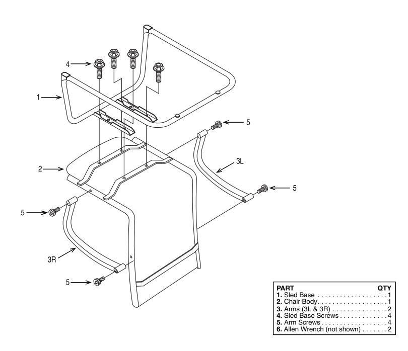
Remove all the parts from carton, separate them into part numbers indicated on the list and make sure part quantities are correct.
