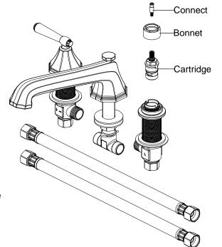
Many of these parts come preassembled. This exploded diagram is to assist in trouble shooting.
