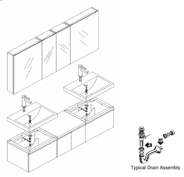
Connect the trap to the drain assembly hand tight to check alignment. It may be necessary to cut off part of the tailpiece ( are "A") or part horizontal leg of the trap (area "B") trap joints for watertight assembly. Connect hot and cold supply lines to the shut off valves. Tighten
