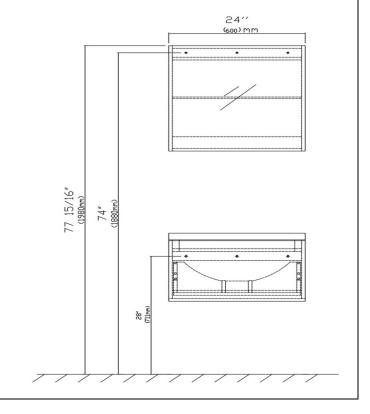
**Step One**: Use the track level bar, tape measure and pencil to mark holes in desired location. Having established the position, use drill to make holes. Use the hammer to insert anchors into the hole and screw in the screws. Finally put the mirror in place.
