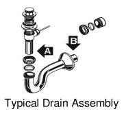
Connect the trap to the drain assembly hand tight to check alignment. It may be necessary to cut off part of the tailpiece (are "A") or part horizontal leg of the trap (area "B") trap joints for watertight assembly. Connect hot and cold supply lines to the shut off valves. Tighten
