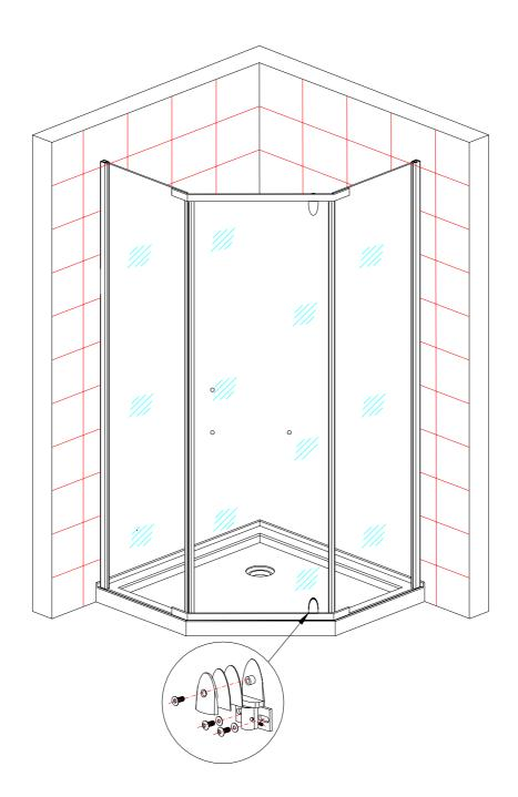
Using the hardware provided install the hinges onto the mounting cross bars.
