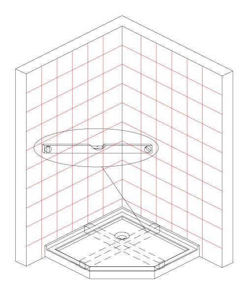
The shower tray needs to sit on a flat level base for proper support. Ensure that the area for the shower tray is properly prepared for installation.
