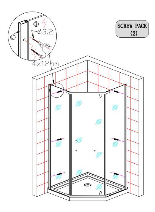
Use a Ø1/8 inch diameter drill bit and drill 3 equally spaced holes along each wall channel on the inside of the shower. Do not drill all the way thru to the other side drill only until the drill bit enters the void in the wall channel. Using the hardware provided secure the fixed glass panel to the wall channel. Repeat on the other side. Decorative covers are also provided to cover the screw heads.
