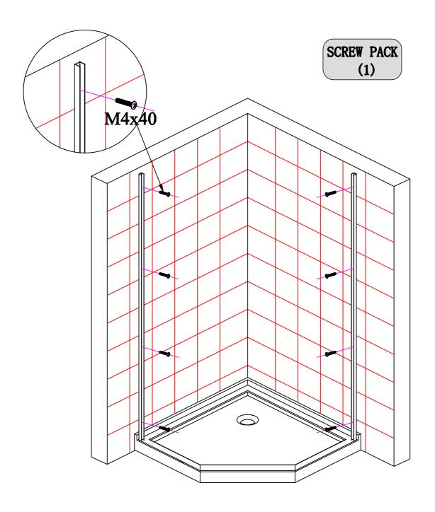
Mount the wall channels to the wall using the screws provided .
