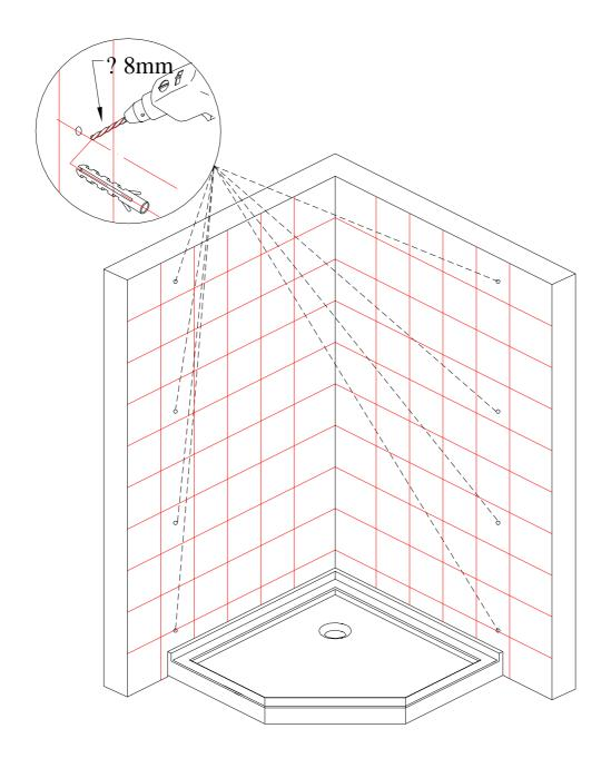
Using the appropriate drill bit for your wall surface drill each hole location with a 5/16" diameter drill bit. Install the plastic wall anchors provided into the drilled holes
