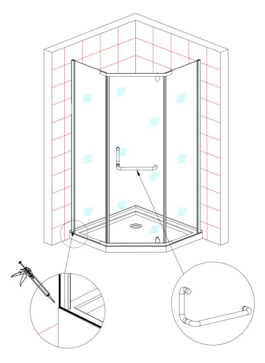
Install the door handle using the hardware provided be sure to use the silicone washer provided between the glass and the door handle to prevent scratching.
