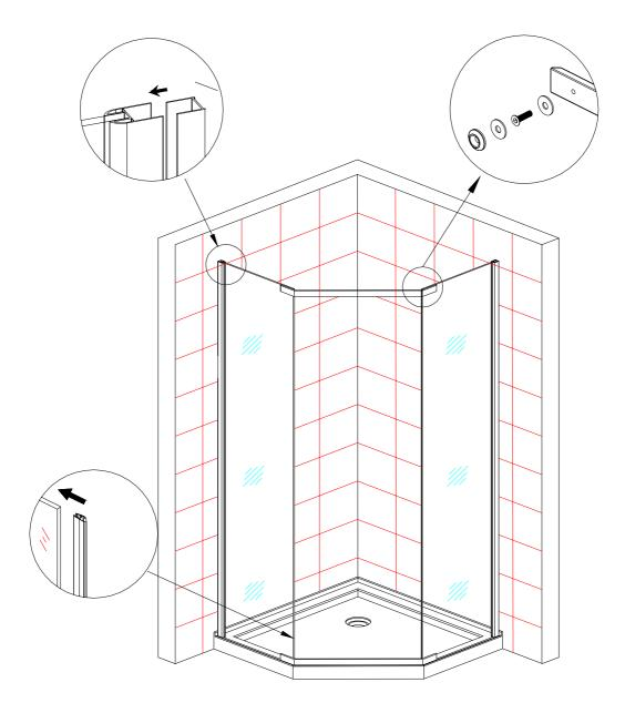
The fixed glass panel has a female channel for the wall channel to slide into. The fixed glass wall channel will install over the mounted wall channel. Slide the fixed glass panel over the mounted wall channel. Repeat installation for the other side.
