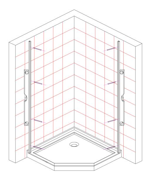
Install all of the wall material or materials you intend to use before installing the wall channels this includes all moisture resistant wall board or rock board, tile, stone or other wall covering.
