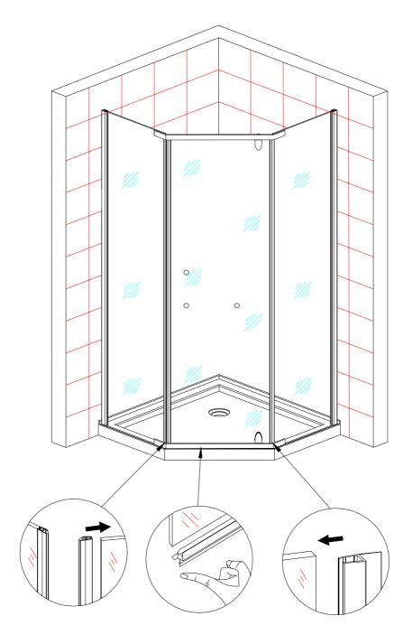
Install the bottom seal and the side magnet seal on the door. Once you have installed all of the seals close to door and ensure a seal is created the entire length of the door. Make adjustments if necessary to the door to create a positive seal.
