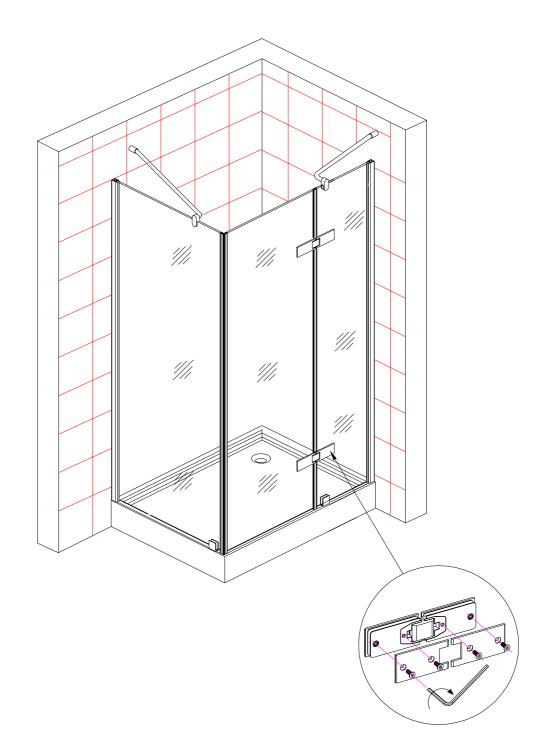
Using the hardware provided install the hinges .
