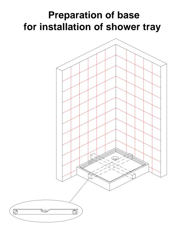
The shower tray needs to sit on a flat level base for proper support. Ensure that the area for the shower tray is properly prepared for installation.
