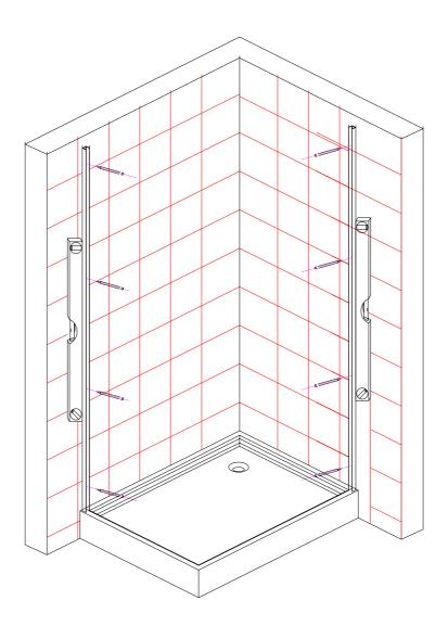
Install all of the wall material or materials you intend to use before installing the wall channels this includes all moisture resistant wall board or rock board, tile, stone or other wall covering.
