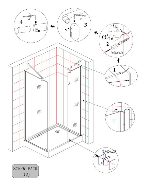
The fixed glass panel has a female channel for the wall channel to slide into. The fixed glass wall channel will install over the mounted wall channel. Slide the fixed glass panel over the mounted wall channel. Repeat installation for the other side.
