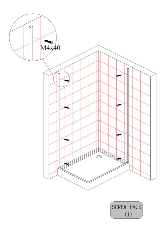
Mount the wall channels to the wall using the screws provided.
