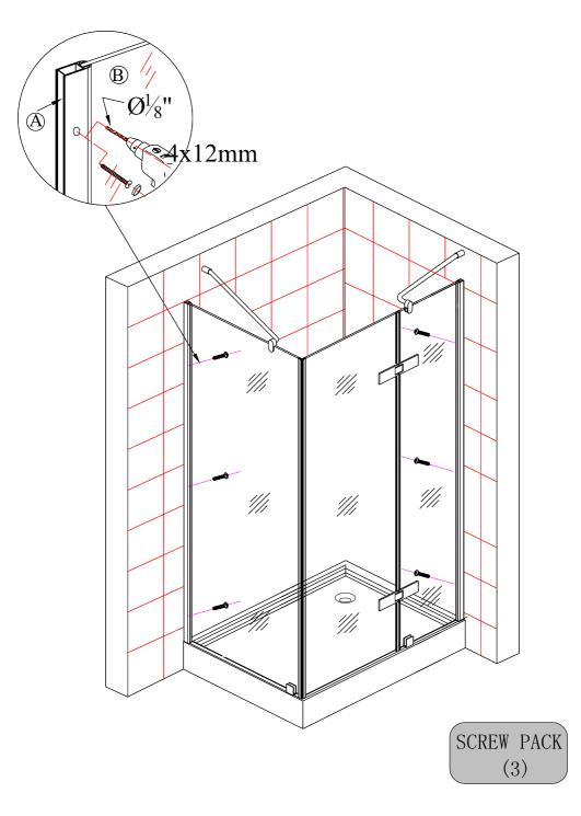
Use a ? 1/8 inch diameter drill bit and drill 3 equally spaced holes along each wall channel on the inside of the shower. Do not drill all the way thru to the other side drill only until the drill bit enters the void in the wall channel. Using the hardware provided secure the fixed glass panel to the wall channel. Repeat on the other side. Decorative covers are also provided to cover the screw heads.
