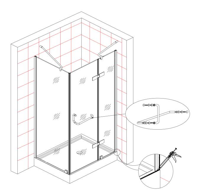
Install the door handle using the hardware provided be sure to use the silicone washer provided between the glass and the door handle to prevent scratching.
