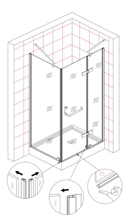
Install the bottom seal and the side magnet seal on the door. Once you have installed all of the seals close to door and ensure a seal is created the entire length of the door. Make adjustments if necessary to the door to create a positive seal.
