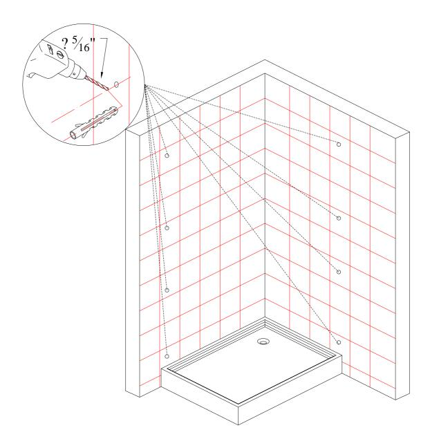
Using the appropriate drill bit for your wall surface drill each hole location with a ? 5/16" diameter drill bit. Install the plastic wall anchors provided into the drilled holes
