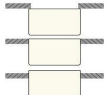
**Step 1: Countertop Cut-Out.** Use the sink upside down to trace the cut out of the countertop. Use precise measurements.
