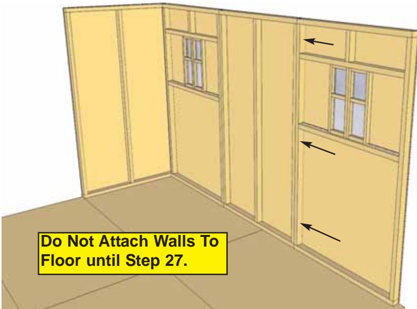
2x3 wall framing flush with outside of plywood.
