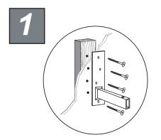
This mounts wall plate must be secured to a stud or other solid surface capable of supporting the total weight of the mount and speaker. Attaching the wall plate to drywall using drywall anchors will decrease the maximum weight handling and is done at the customers own risk.
