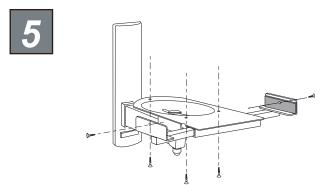
in order to maintain maximum safety it is necessary to use the small security screws.
