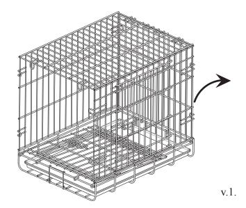
Unfold front panel and firmly pull into place.
