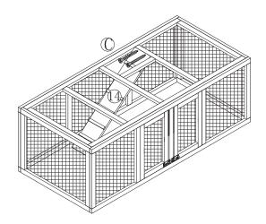
Turn the structure 180°. Align parts (5), (6), and (7) on top of part (4). Connect parts (5), (6) and (7) using screws (B). Do not tighten completely.
