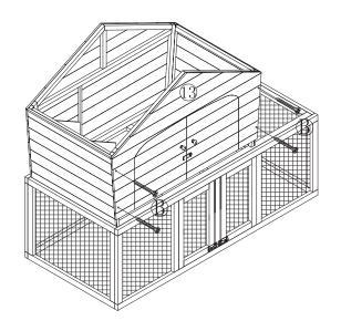
Secure part (16) onto the structure using screws (A).
