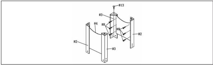
3. Attach assembled LEGS to TABLE BODY #1 with BOLT #6 and FLAT WASHER #7. Note: The table is assembled upside down.
