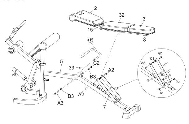
Insert the short end of the Seat Adjustment Bar (16) into Main Frame (5) as shown.
