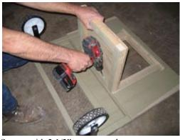
Secure with 2 1/2" screws as shown.
