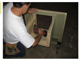
Make sure the opening is flush on the inside and secure with 2 1/2" screws.
