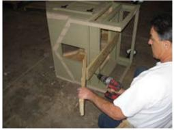
Next insert 2 1/2" screw from the bottom up as shown in predrilled holes.
