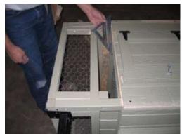
Make sure the floor is flush with the bottom of the wall as shown.
