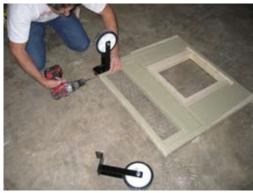
Fasten wheels on the bottom as shown with 2 1/2" deck screws.
