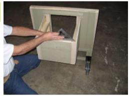
Install the back panel. Make sure the top is flush.
