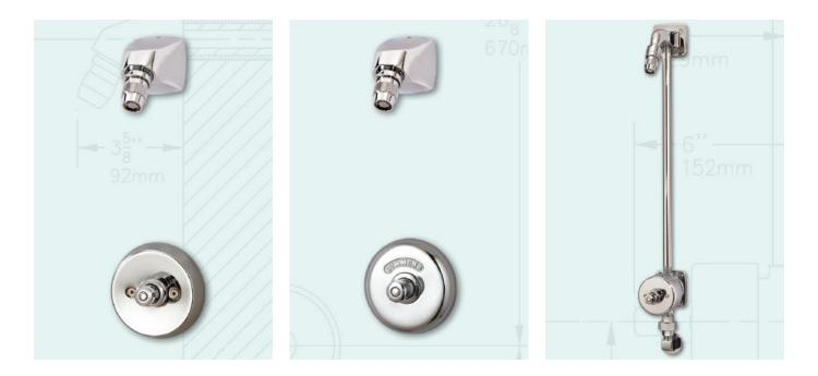
**3-310** SHOWEROFF concealed metering shower valve with integral stop and 1/2" IPS **back connections** (model 4-427). Fre-Flo institutional shower head with adjustable spray (model 4-295B). All mounting fasteners for valve and head are vandal-resistant recessed hex socket type.
