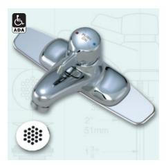
**S-60-G-H-DP** SCOT metering/temperature selection lavatory faucet with blade type handle and adaptor plate drilled on 8" centers. Cast brass slow-closing lavatory faucet to meter and mix hot and cold water supply. Temperature limit stop to adjust outlet temperature. Time limit stop to adjust flow time. Includes two (2) in-line check/screen assemblies. Spray outlet with 0.5 gpm flow rate. Vandal resistant. Grid strainer drain assembly.
