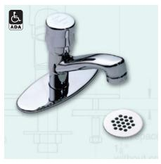
**S-72-G** Metering faucet with deck plate to accommodate 4" center, 3 hole mounting sink basins. Faucet to meter a single cold, hot or tempered water supply. Adjustable time limit stop to adjust flow time. Vandal resistant 0.5 gpm spray outlet. Grid strainer drain assembly.
