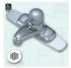
**S-61-G-DP** Metering faucet with adaptor plate drilled on 8" centers. Cast brass slow-closing lavatory faucet to meter a single tempered water supply. Time limit stop to adjust flow time. Includes in-line check/screen assembly. Spray outlet with 0.5 gpm flow rate. Vandal resistant. Grid strainer drain assembly.
