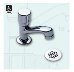
**S-71-G** Single Post Metering faucet to meter a single cold, hot or tempered water supply. Adjustable time limit stop to adjust flow time. Vandal resistant 0.5 gpm spray outlet. Grid strainer drain assembly.
