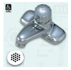
**S-61-G** Metering faucet. Cast brass 4" centerset slow-closing lavatory faucet to meter a single tempered water supply. Time limit stop to adjust flow time. Includes in-line check/screen assembly. Spray outlet with 0.5 gpm flow rate. Vandal resistant. Grid strainer drain assembly.
