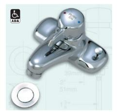
**S-60-P-H** SCOT metering/temperature selection lavatory faucet with blade type handle. Cast brass 4" centerset slow-closing lavatory faucet to meter and mix hot and cold water supply. Temperature limit stop to adjust outlet temperature. Time limit stop to adjust flow time. Includes two (2) in-line check/screen assemblies. Spray outlet with 0.5 gpm flow rate. Vandal resistant. Pop-up drain assembly.
