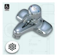
**S-60-G-H** SCOT metering/temperature selection lavatory faucet with blade type handle. Cast brass 4" centerset slow closing lavatory faucet to meter and mix hot and cold water supply. Temperature limit stop to adjust outlet temperature. Time limit stop to adjust flow time. Includes two (2) in-line check/screen assemblies. Spray outlet with 0.5 gpm flow rate. Vandal resistant. Grid strainer drain assembly.
