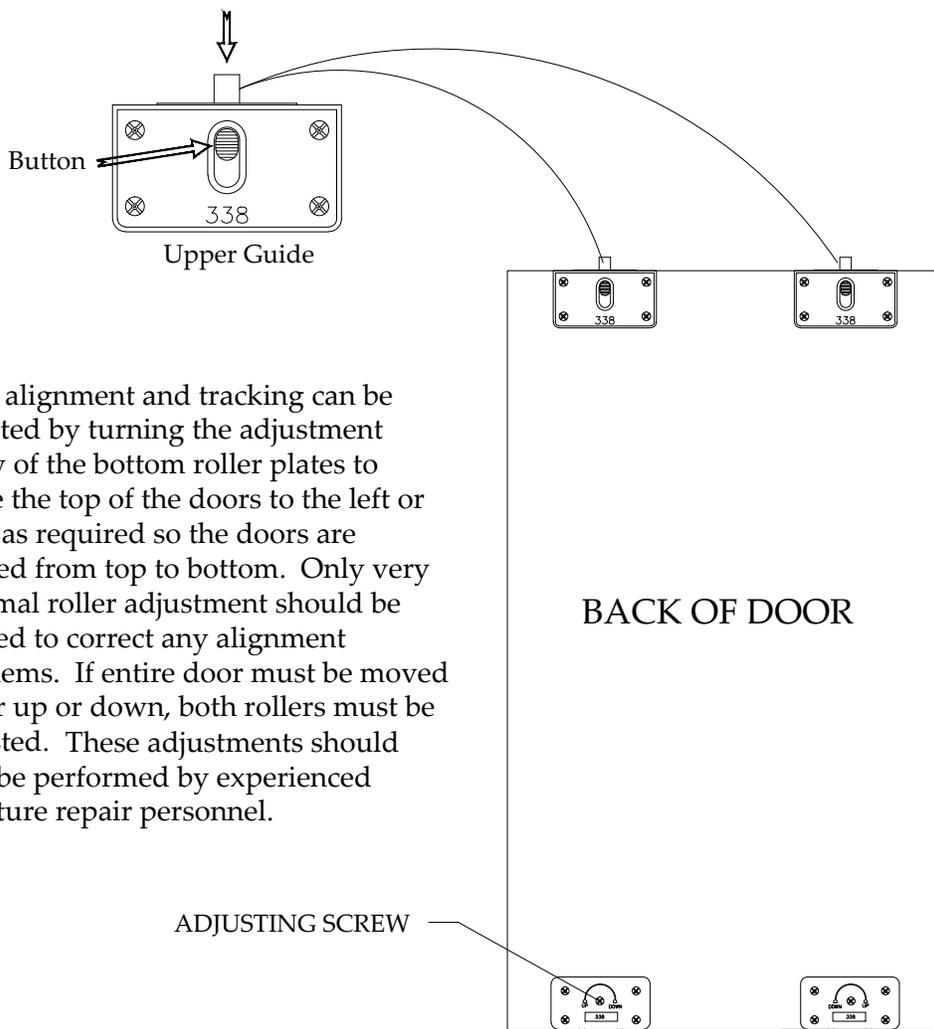
Door alignment and tracking can be adjusted by turning the adjustment screw of the bottom roller plates to move the top of the doors to the left or right as required so the doors are aligned from top to bottom. Only very minimal roller adjustment should be needed to correct any alignment problems. If entire door must be moved either up or down, both rollers must be adjusted. These adjustments should only be performed by experienced furniture repair personnel.
