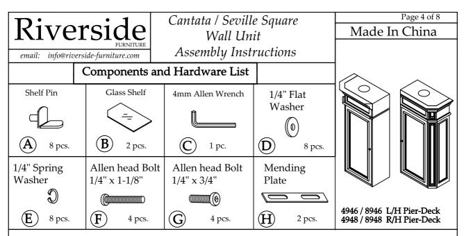
**Step 1:** Remove the Screws attaching the Top Panel and lay the Top Panel and Screws aside, until the Bridge is connected to the Piers. Assemble the Top Crown using the Allen head bolt (F), Spring Washer (E) and Flat Washer (D). Take care running the wiring for the lights so that it does not get pinched or stressed. Tighten the Allen Bolts using the Allen Wrench (C).
