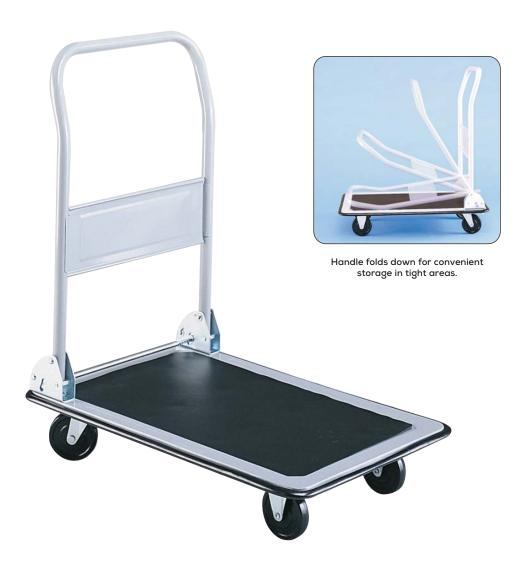
Industrial strength and quality at a surprisingly low price. Solid, all-welded steel frame with 400 lb. (4072) or 500 lb. (4063) weight capacity. Features include a large platform with anti-skid mat and big 4" casters— two stationary and two swivel for easy maneuverability on any surface, folding handle for easy storage and %" wrap-around vinyl bumper to protect doors and furniture from damage. Strong, chip-resistant light Gray enamel finish with black vinyl trim.
