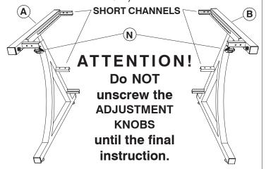
Place the (A) Left Frame Assembly on a protected surface with the short channels upward. Insert the (H) Tube Plugs if they are not already installed on the tube ends. Insert the (D) Levelers. Repeat with the (B) Right Frame Assembly.
