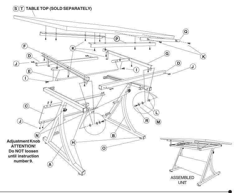
Locate the (A) Left Frame Assembly (the short channels will be on the right side of the frame), and the (B) Right Frame Assembly (the short channels will be on the left side of the frame).
