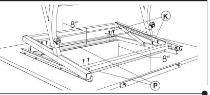
Lower the Drawing Board to the flat position by raising the (E) Lift Bar upward with one hand while easing the board downward with the other hand. (see inset)
