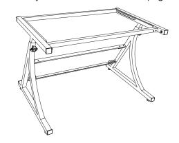
Place one (L) Nylon Spacer on the pin. Insert the (G) Support Channel onto the pin. Place one (L) Nylon Spacer and one (M) Washer on the pin and fasten securely using one (R) Short Pan Head Machine Screw. Repeat for the other support channel and frame.
