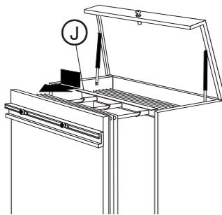
Insert the (J) Drawing Selector behind the desired drawing so the notches ride on cabinet posts. Use the Selector to move the groups of drawings from posts to pins.
