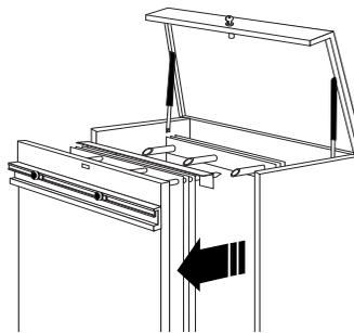
When selected drawings are on the pins, roll the entire drawer away from the cabinet **as far as it will go**, disengaging the pins from the posts.
