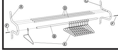
NOTE: due to the potential weight of a full rack, we do not recommend mounting to a drywall (wallboard) surface unless both end brackets are fastened into wood or metal studs.
