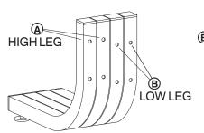
Identify the two types of legs: the (A) High Leg has its mounting holes 1/2" closer to the top of the tubing than the (B) Low Leg.
