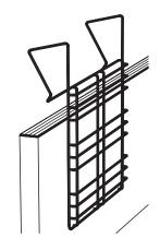
Place Mini-GridWall hanger over office panel, as shown at left (you may have to spread the wire hanger slightly for thicker panels, but take care not to over-bend).
