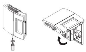
2 Connect the thermostat wires to the line wires and to the load wires using solderless connectors for copper wires.
