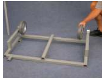
Lay base down as pictured and bolt on both wheels securely.
