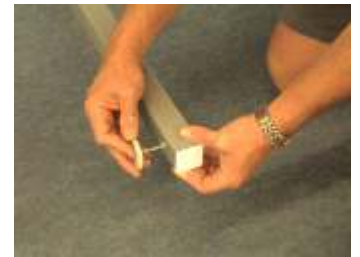
Screw each leveler all the way in. Do not over tighten.
