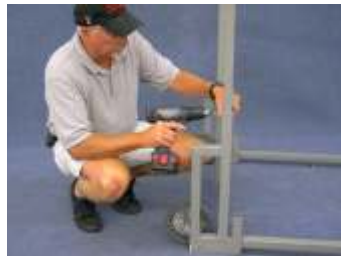
Using drill and socket cap screw provided, screw in the 4 self tapping screws.
