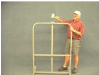
Use rubber mallet to tap down until it bottoms out.
