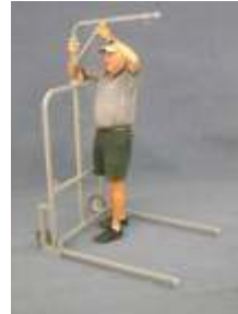
Insert Boom into slot on top of the M-Shaped piece. Make sure it bottoms out.
