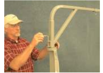
You can change positions of the boom by lifting pin
