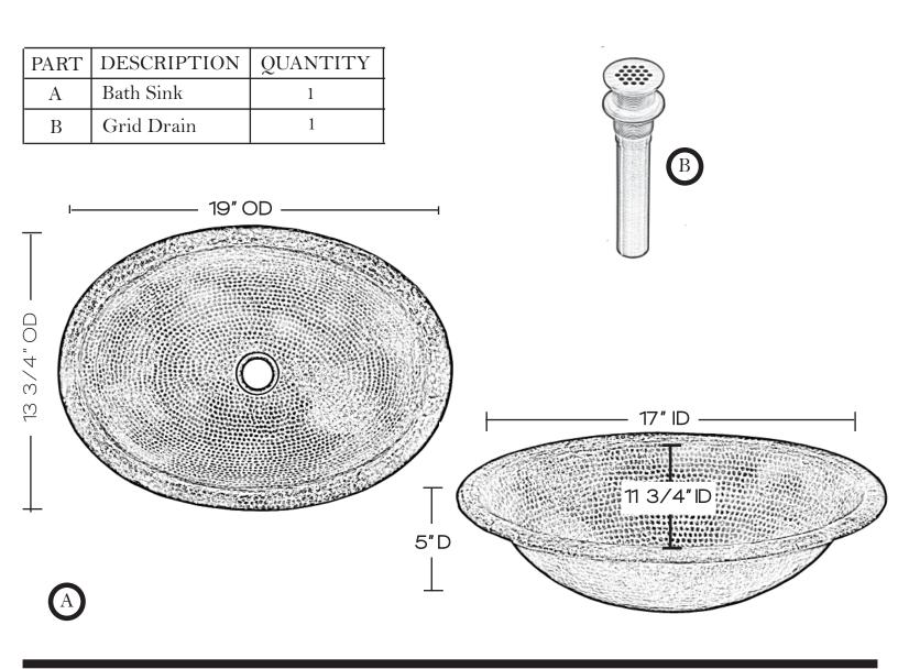
Your copper sink A is handmade and therefore a work of art. Each sink is unique and can vary 1/4" in either direction. We highly recommend waiting to receive your sink before cutting your counter top.
