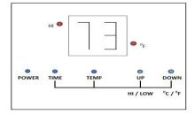
5) Press the HI/LOW/UP button to switch from HI (rated at 1500W) to LOW (rated at 750W). The default setting is HI.
