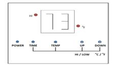
5) Press the HI/LOW/UP button to switch from HI (rated at 1500W) to LOW (rated at 750W). The default setting is HI.
