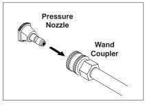
**STEP 7:** Pull spring-loaded collar of the wand coupler back to insert your choice of pressure nozzle.
