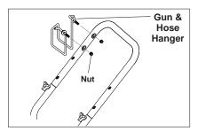
**STEP 3:** Attach the Gun & hose hanger and insert nuts from inside. Tighten nuts.
