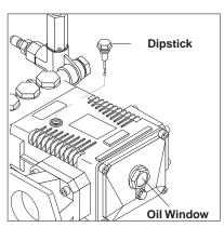
STEP 2: Remove shipping cap and install oil dipstick. Check pump oil level by using dipstick or observe oil level in oil window (if equipped). Use 40 wt. non detergent oil. The Legacy Axial Pump does not require maintenance. Attemping to check oil on this pump may damage it and will void your pump warranty.
