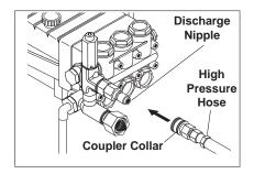
**STEP 9:** Connect the high pressure hose to the discharge nipple. Push coupler collar forward until secure.
