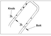
**STEP 2:** Insert the carriage bolt through the holes from the back of the unit and attach a knob from the front of the machine. Tighten Knobs with by hand.
