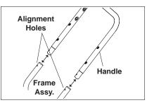
**STEP 1:** Attach the handle to the frame of the pressure washer. **Note**: It may be necessary to move the handle supports from side to side in order to align the handle so it will slide over the frame supports.
