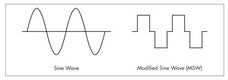
This modified sine wave has a root mean square (RMS) voltage of 115 volts. Most ordinary AC voltmeters are calibrated to read "average" voltage and assume that the AC waveform will be a pure sine wave. These meters will not correctly read MSW voltage, and will display about 20 to 30 volts too low. Any multi-meter identified as "TRUE RMS" will accurately read MSW correctly.
