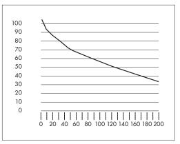
©2013 Wagan Corporation. All Rights Reserved. Wagan Tech and *wagan.com* are trademarks used by Wagan Corporation. The curve can be applied to any lead acid battery under load providing that it has an AH rating at the 20 hour rate.
