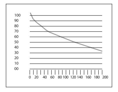
The curve can be applied to any lead acid battery under heavy load providing that the battery has an AH rating "at the 20 hour rate".
