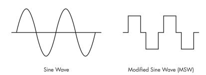
MSW has a root mean square (RMS) voltage of 115 volts. Most ordinary AC voltmeters are calibrated to read "average" voltage and assume that an AC waveform is a sine wave. Average reading meters do not correctly read MSW voltage, and will display 20 to 30 volts too low. Multi-meters identified as "TRUE RMS" will accurately read MSW voltage.
