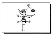
Apply a small bead of Plumber's putty to underside of flange (1). Insert body (2) into sink. Screw flange (1) into body (2). Pivot (3) must face faucet. Pull assembly down firmly and hold in place. DO NOT TWIST. Tighten nut, washer & gasket (4), clean off excess Plumber's putty.
