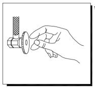
Shut off water supply at angle stop. Remove old faucet. Clean sink surface in preparation for new faucet.
