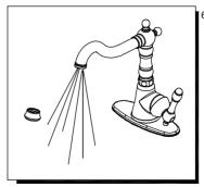
6. Important: After installation is completed, remove aerator. Turn on water supply and allow both hot and cold water to run for at least one minute each. While water is running, check for leaks. Replace aerator.
