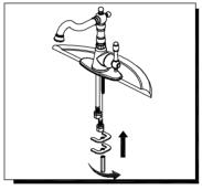
From underside, assemble rubber Washer metal washer and mounting nut onto the thread rod and tighten mounting nut. Do not overtighten .
