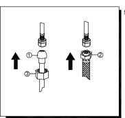
5.Make Connections to water lines: Choose hook-ups for 1/2" I.P.S. connections: (1) Ball nose riser (3/8" O.D. copper tubing), or (2) 1/2" I.P.S. faucet connector .Use the enclosed coupling nuts (3) with the ball nose risers (1). Use two wrenches when tightening. Do not overtighten.
