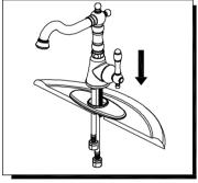
3.Place new faucet hoses and thread rod through the center hole of sink.
