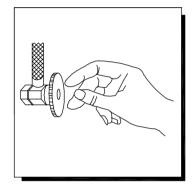
1. Shut off water supply at angle stop. Remove old faucet. Clean sink surface in preparation for new faucet.
