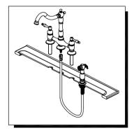
Insert sprayer hose down through support and sink. Attach sprayer hose to sprayer hose nipple.
