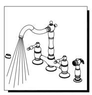
Important: After installation is completed, remove aerator. Turn on water supply and allow both hot and cold water to run for at least one minute each. While water is running, check for leaks. Replace aerator.
