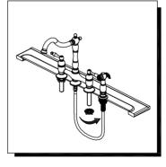
4. From under sink, threads mounting nuts onto faucet. Tighten mounting nuts.
