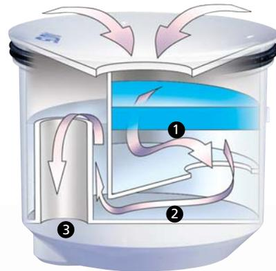
The cartridge acts as a funnel directing flow through the liquid sealant ①, preventing any odors from escaping. Next, the cartridge collects sediment ②, allowing the remaining waste to pass freely down the drain ③.
