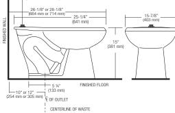
NOTE: All vitreous china dimensions shown in these drawings are nominal. Dimensions can vary within the tolerances established in the governing ASME A112.19.2/CSA B45.1 standard. Please take this into consideration when planning rough-in and plumbing layouts.
