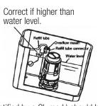
With the valve installed, the critical level mark on the fill valve (identified by a CL mark) should be at least 1" (25 mm) above the top of the water level. Water temperature should be in the range of 45° F (2° C). Water supply static pressure range: 20psi-80psi.
