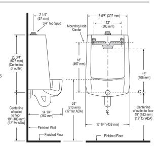
NOTE: All vitreous china dimensions shown in these drawings are nominal. Dimensions can vary within the tolerances established in the governing ASME A112.19.2/CSA B45.1 standard. Please take this into consideration when planning rough-in and plumbing layouts.
