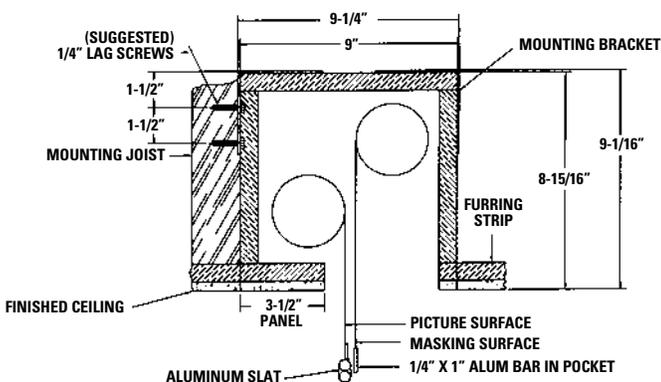
Offset mounting, recessed above ceiling. May be adapted for 1/4" paneling for ceiling.
