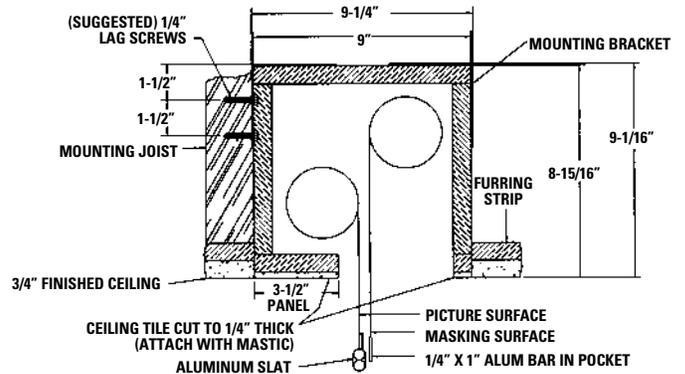
Offset mounting, recessed above ceiling. For plaster, dry wall, tile or paneling. Bottom of case painted same finish as ceiling.
