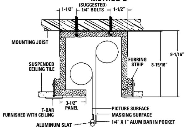
Flush mounting, recessed above ceiling. For use with dropped ceiling. May also be adapted for use with acoustical or other ceiling 3/4" thick but cut to 1/4" thick under screen case and panel.
