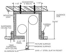
Flush mounting, recessed above ceiling. For use with dropped ceiling. May also be adapted for use with acoustical or other ceiling 34" thick but cut to 14" thick under screen case and panel.
