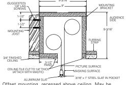
Offset mounting, recessed above ceiling. May be adapted for ¾" ceiling, but cut to ¼" thick under screen case and panel.
